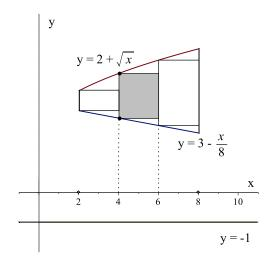
Find the volume of the shape obtained by revolving the shaded rectangle about the line y = -1.
